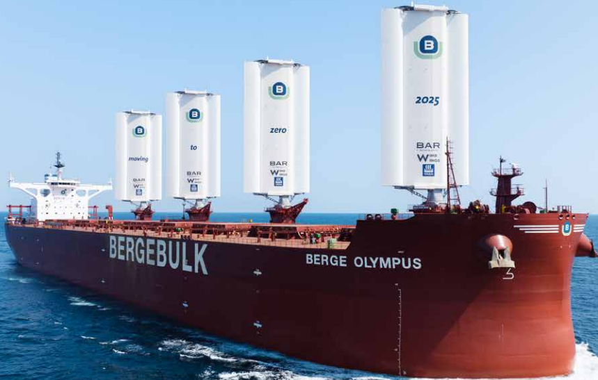
Berge Olympus equipped with BARTech WindWings
